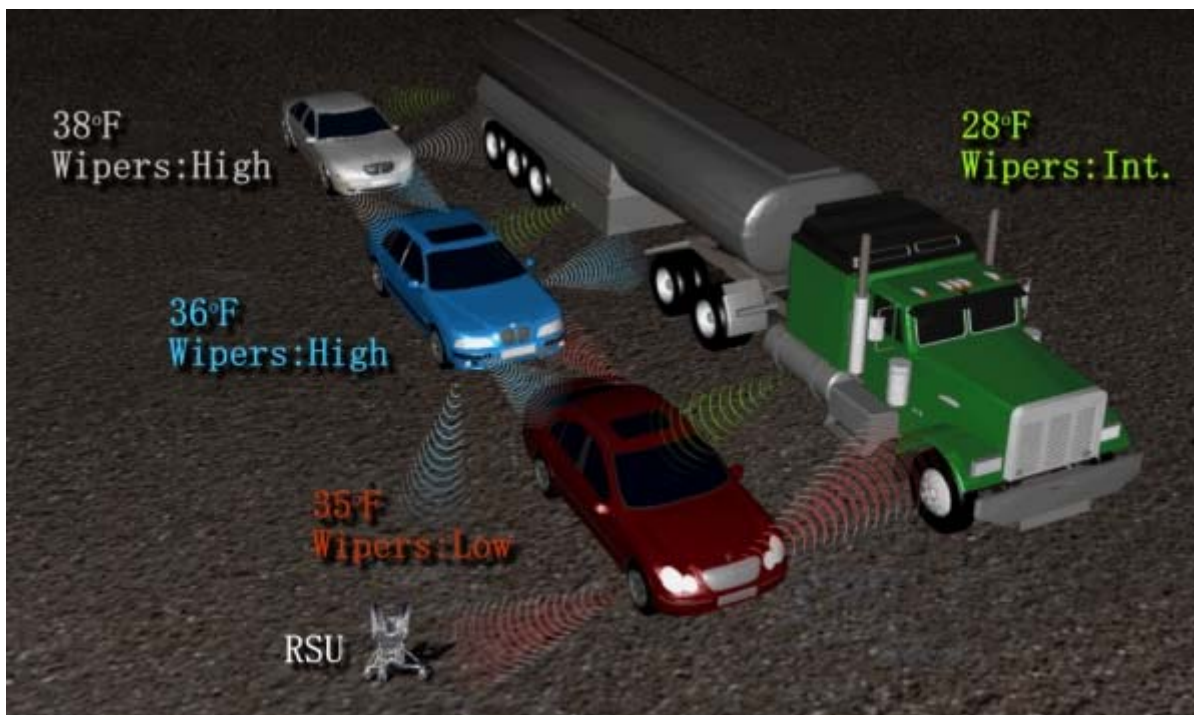
Figure 5: Concept of Vehicle Infrastructure Integration (Source: US DOT, 2006).
